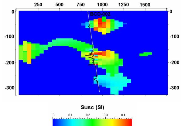
**Figure 13:** EW cross-section (7661425mN, marked in Figure 11) illustrating the susceptibility model after combined geometry and property inversion. Downhole susceptibility logs shown in black. Drill hole BCD-002 is oblique and has been projected onto the section. Vertical exaggeration 1:3.
