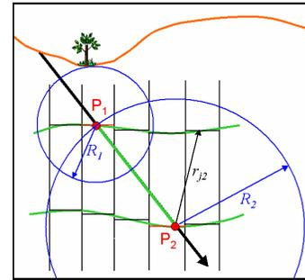
**Figure 4:** Schematic section showing radius of influence around pierce points, within which geometry changes are damped during inversion. In VPmg,  $R$  is defined as the lesser of depth and distance to nearest pierce point.
