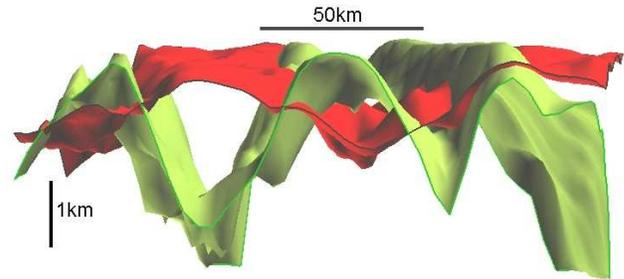
**Figure 10:** Perspective view of inferred basement surface, comparing the results after constrained (red) and unconstrained (green) geometry inversion.
