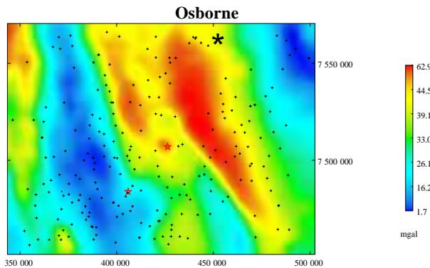
**Figure 6:** Free-air gravity image, Boulia 1:250,000 sheet, Queensland. Drill holes intersecting basement are marked as red stars. Basement depths were 1300m (central) and 530m (SW). Water bore locations are marked with black crosses. (Data courtesy Queensland Department of Natural Resources and Mines).
