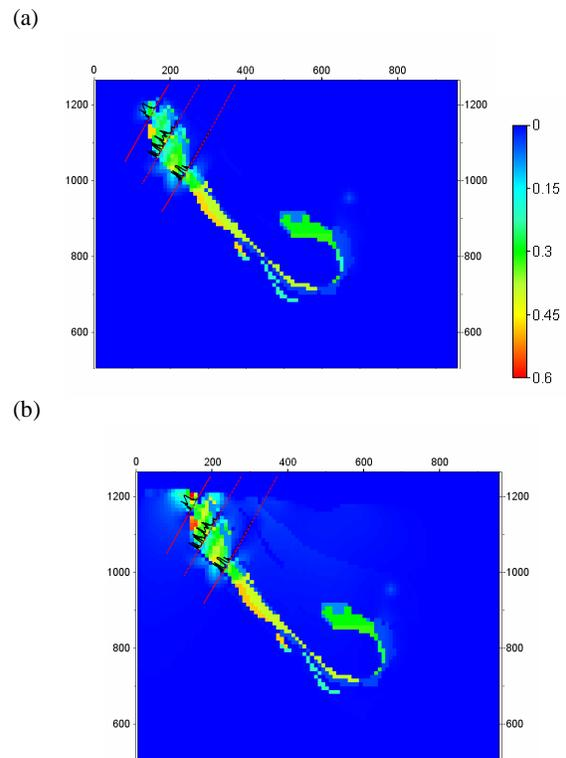
**Figure 20:** Cross-section along 4795N (marked in Figure 16), coloured by susceptibility (SI). Core susceptibility logs (black) and corresponding drill holes (red) superimposed. (a) Starting model for heterogeneous unit inversion, after blending of homogeneous unit susceptibilities with drill hole susceptibilities. (b) Model after heterogeneous unit inversion. Susceptibility has spread into host units, especially into the footwall gneiss at shallow depths.
