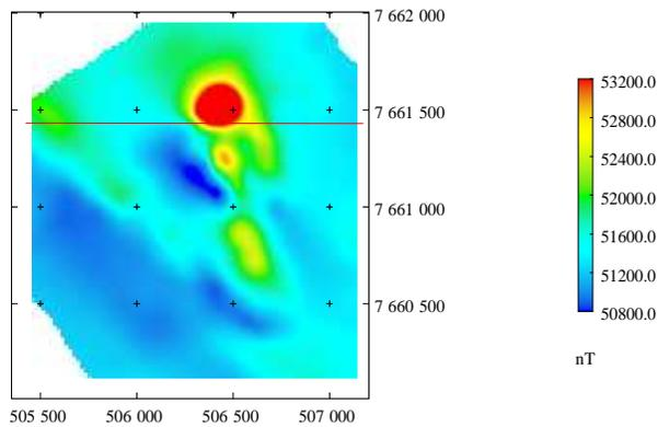
**Figure 11:** Bull Creek total magnetic intensity image, based on ground readings. (Data courtesy Exco Resources).
