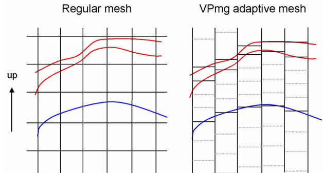
**Figure 2:** Schematic model sections illustrating the differences between a conventional fixed mesh (left) and the deforming mesh implemented in VPmg. Sub-cells (dotted boundaries) can differ in size from one rock type to another.
