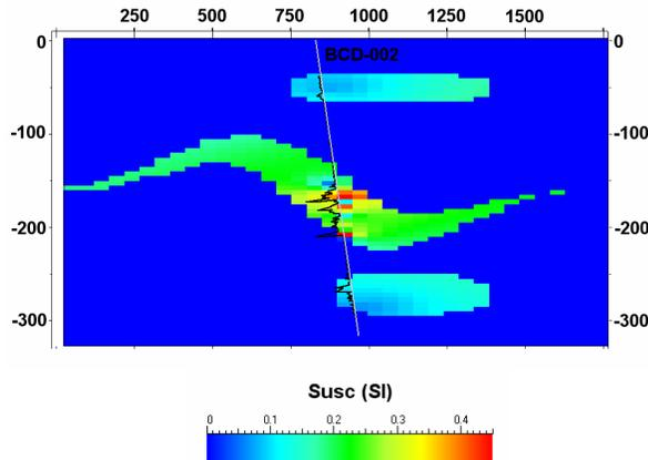
**Figure 12:** EW cross-section (7661425mN; marked in Figure 11) illustrating the three susceptible bodies in the starting model in relation to the BCD-002 drill hole. Downhole susceptibility logs shown in black. Drill hole is oblique and has been projected onto the section. Vertical exaggeration 1:3.
