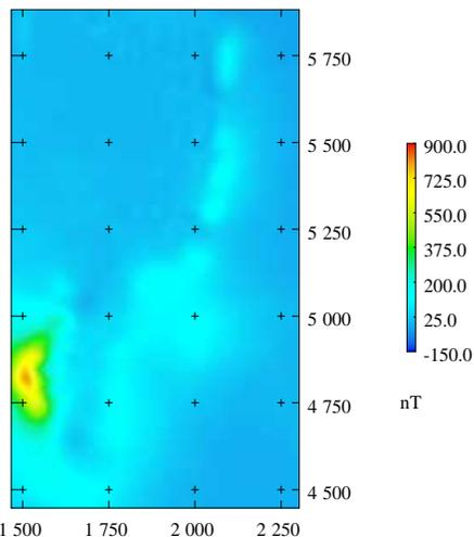
**Figure 22:** Residual TMI after heterogeneous property inversion if susceptibility is fixed at zero in gneiss. The amplitude of the crescent-shaped residual anomaly is ~700 nT.
