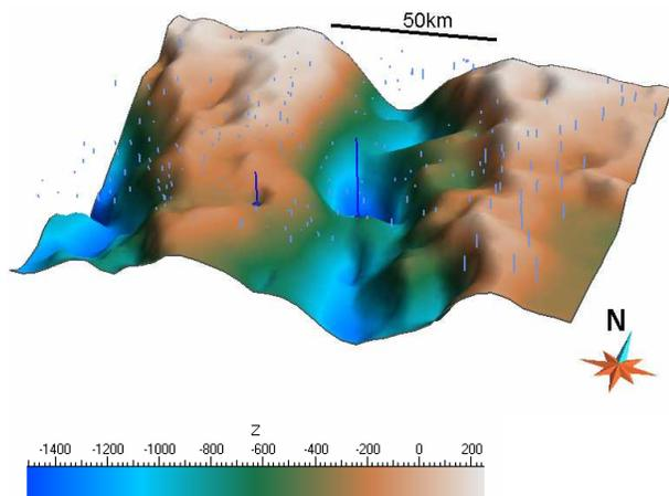
**Figure 9:** Perspective view of the basement contact after constrained geometry inversion, with water bores (blue) and deep drill holes (purple) superimposed. Colour indicates elevation (mASL).
