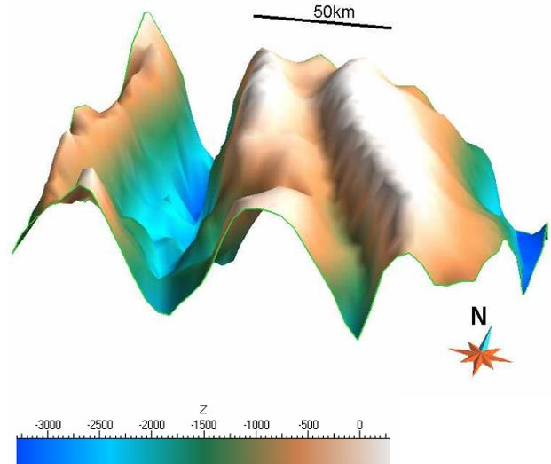
**Figure 7:** Perspective view of the basement surface after unconstrained geometry inversion. The colour depicts elevation (mASL). Vertical exaggeration 1:20.
