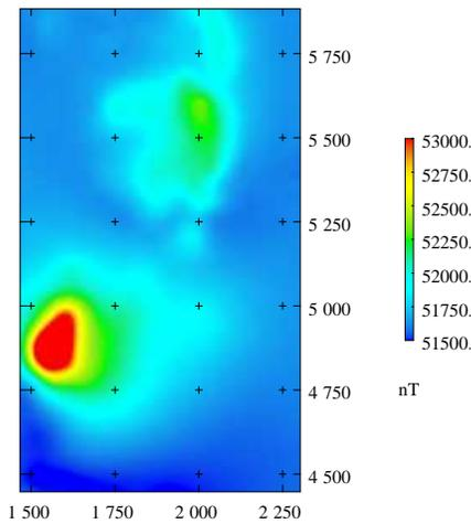
**Figure 21:** Computed TMI after heterogeneous unit inversion. Final RMS misfit is 9nT.
