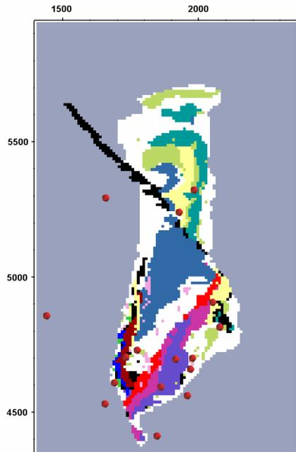
**Figure 17b:** Horizontal section at RL 895m, illustrating Cannington geology. Colours refer to mineralisation types (Figure 17a). Red dots mark intersection points, at this level, for holes from which susceptibility readings were derived. NW-SE striking Treppel Fault zone shown in black.
