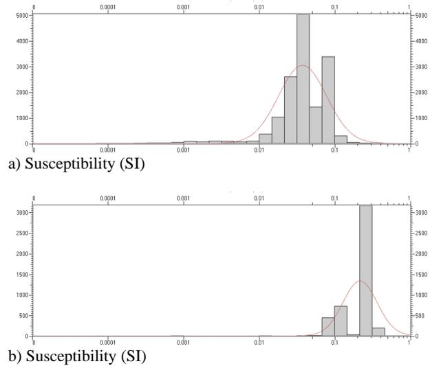
**Figure 23:** Susceptibility histograms for (a) Broadlands and (b) Burnham mineralisation after inversion based on 14721 and 4582 10m cells respectively. These histograms refer to all model cells classified as either Broadlands or Burnham.
