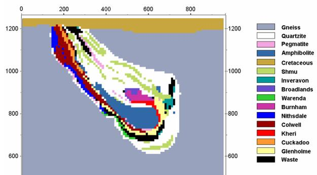
**Figure 17a:** EW cross-section 4795N, illustrating Cannington geology. Red line in Figure 16 marks the section location. Colours refer to mineralisation types. Horizontal axis represents distance from western edge of model.
