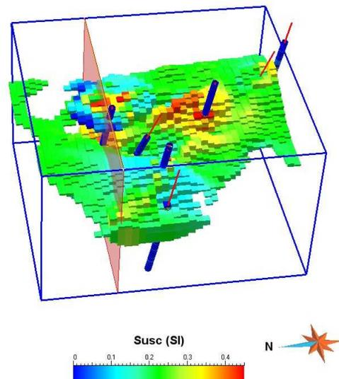
**Figure 14:** Cells within the magnetic bodies, coloured by susceptibility, after combined geometry and property inversion. Drill holes with susceptibility measurements are shown. The location of the cross-section depicted in Figures 12 and 13 is indicated by transparent plane.
