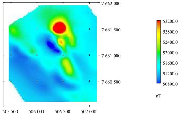
**Figure 15:** Computed TMI response of the Bull Creek model after combined geometry and property inversions.
