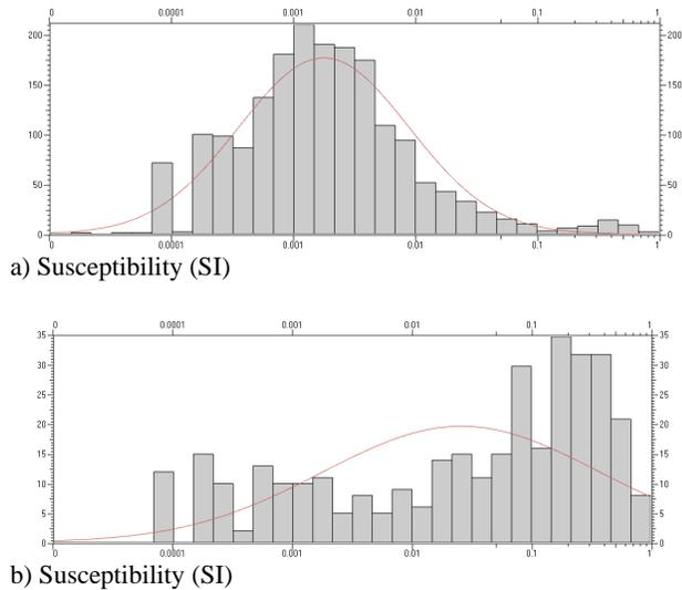
**Figure 18:** Histograms for drill hole susceptibility data (1m intervals) for (a) Broadlands and (b) Burnham mineralisation, based on 1875 and 345 readings, respectively.
