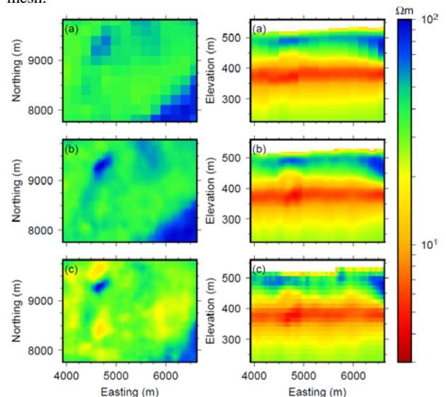
**Figure 3:** Comparison of (left) plan-view and (right) cross sections for the (a) coarse and (b) fine pseudo-3D models, and (c) the 3D recovered model. The left-hand figures are at an elevation of 465 m. The right-hand figures, at a northing of 8400 m, are vertically exaggerated to show variations in the resistivity with depth.
