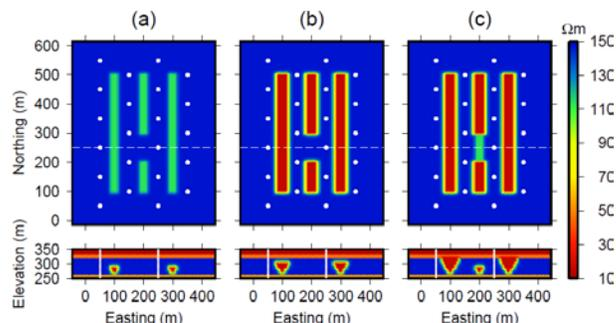
**Figure 5:** True resistivity model showing three steam chambers at different time steps.
