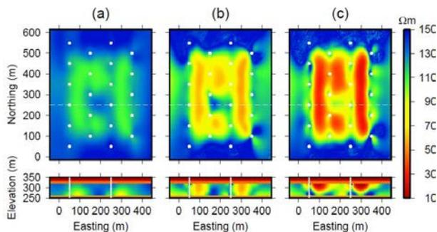
**Figure 7:** Recovered resistivity models from inverting EM data at different time steps.
