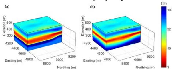
**Figure 4:** a) A semi-synthetic McMurray Formation and Devonian basement are added to the 3D recovered model using borehole data. b) Inversion of surface EM data recovers the McMurray Formation.
