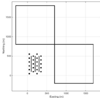
**Figure 6:** Monitoring survey using two large inductive transmitters at the surface and borehole receivers near the SAGD well pad.
