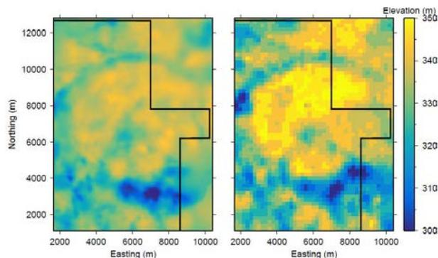
**Figure 2:** Top of the McMurray Formation based on (left) seismic data and well logging and (right) the inversion of airborne EM data.
