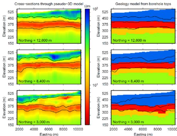
**Figure 1:** (left) Cross-sections through the pseudo-3D model from inverting airborne EM data with an interpretation of the geologic layers; (right) Interpretation from EM data overlaid onto geologic model from borehole data. Note that the figures are vertically exaggerated to show variation in the resistivity with depth.
