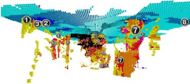
**Figure 1:** Oblique-view looking north of the targets defined by the SGS Geostat team for the 2016 Integra Gold Rush Challenge showing 50 m wide blocks colour-coded by exploration prospectivity: hotter colours are more likely to host gold mineralization. Numbers show the individual targets that were vetted and put forward by the team. The black shapes near the center of the image are the underground workings from Integra Gold Corp’s historic Sigma-Lamaque gold mine.
