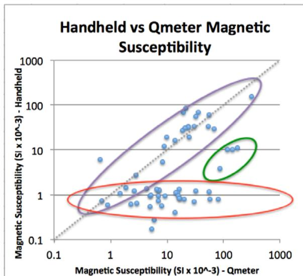
**Figure 6:** Comparison of instrument magnetic susceptibility values (log-scale). Ellipses show: correlating population (Group 1 - purple); effects of remanence and related anisotropy (Group 2 - red); and weathered and ferruginised samples, visible Po content, or proximal to shear zone (Group 3 - green). A dashed line shows hypothetical equal values.
