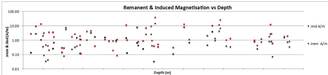
**Figure 3:** Remanent (Jrem) and induced (Jind) magnetisation intensities vs. relative depth.
