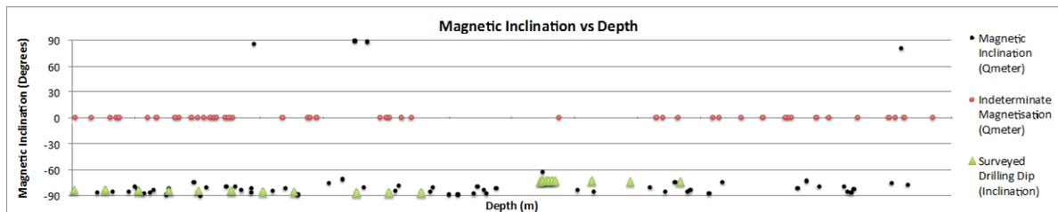
**Figure 4:** Magnetic inclination vs. relative depth. Null values (red) show samples with unreliable magnetic moments due to a lack of magnetic mineral content.
