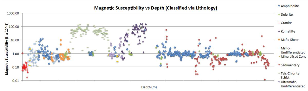
**Figure 1:** Magnetic susceptibility (log-scale) vs. relative depth, classified via the geologist’s lithological log. Due to a requirement of commercial confidentiality, drill-hole ID and actual depths have been omitted. The horizontal scale is therefore a relative depth. Tick marked intervals are 100 m.
