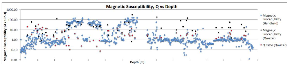
**Figure 5:** Magnetic susceptibility (log-scale) vs. relative depth. Qmeter derived magnetic susceptibility data and Q data are overlain.
