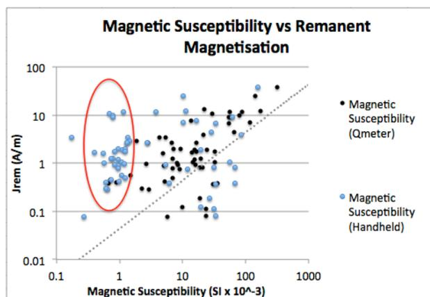
**Figure 7:** Remanent magnetisation intensity vs. magnetic susceptibility data (both log-scale). A slope of unity, as shown by a dashed line, divides the plot between  $Q > 1$  (above the line), and  $Q < 1$  (below the line). Red ellipse is coincident with that in Figure 6.
