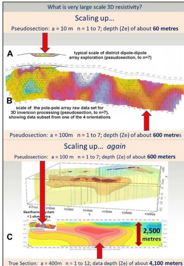
Figure 3: VLS 3D E-SCAN data is acquired by scaling up the electrode grid spacing as needed. No transition to MT data is ever required.
