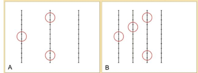
**Figure 1:** Anomalies on lines that are too widely separated (a) and on closer lines (b) that support an objective interpretation by geoscientists, and more importantly, by computers.
