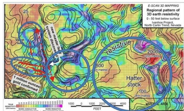
**Figure 14:** From the 3D resistivity inverted model, this plan view at surface shows the Gwenivere and Clementine vein systems, containing >1 million ounces of gold, shown in red at left.
