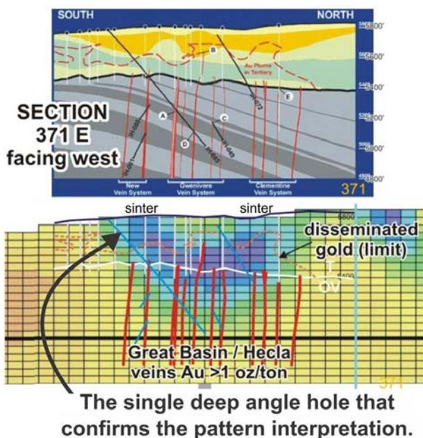
**Figure 13:** Geophysically undetectable feeders in the basement.
