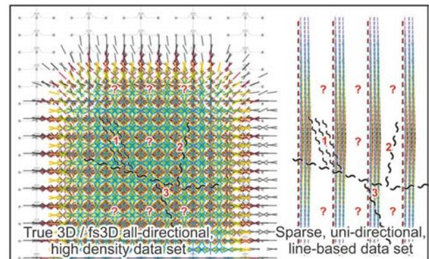
**Figure 2:** True 3D field data sampling vs line-based survey sampling with a depth colour coded tick mark placed at each nominal reading position.
