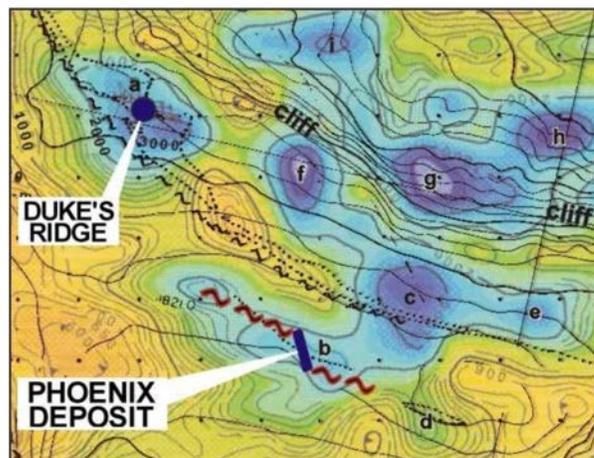
Figure 4: 3D Resistivity inverted model plan view showing high resistivity (blue) anomalies associated with silicic alteration haloes over an 1100 m by 800 m area of Toodoggone volcanics, in central BC.
