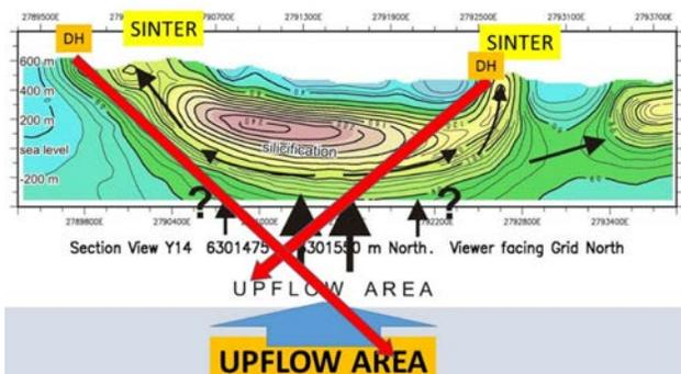
**Figure 10:** Drilling to test real feeder location, rather than the potential drilling configuration displayed in Figure 8.
