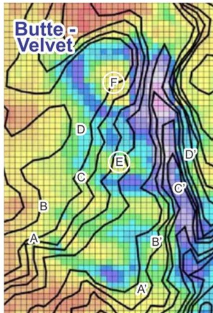
**Figure 16:** Surface traces of U-shaped elevated resistivity for the several parallel U-shaped patterns of Figure 15.
