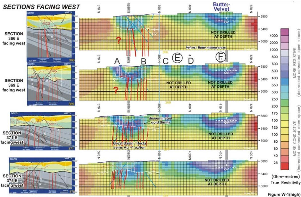
**Figure 15:** The sequence of sections illustrates the linear continuity of the pattern of deep silica precipitation and the lateral (N-S) diversion of upward fluid flow along the Gwenivere-Clementine fault system (at left). Circular patterns located at Butte-Velvet to the north had not been drilled at the time of creation of this circa-2000 3D imagery.
