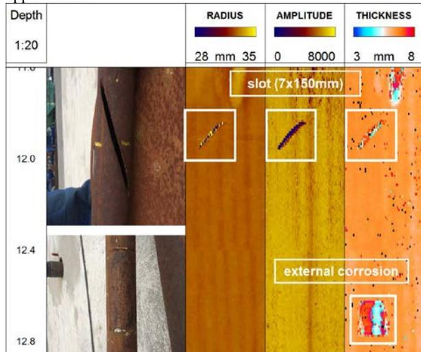
**Figure 3:** Cased hole application in a 2 7/8 inch (73 mm) test tubing.
