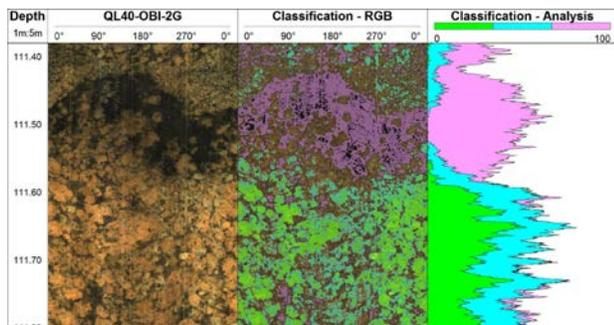
**Figure 2:** High resolution images of optical imaging tools enable mineralogical analysis (e.g. the colorimetry method).
