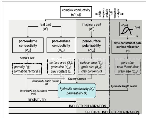
**Figure 7:** Flowchart showing how SIP methodology may be used to determine hydraulic conductivity.
