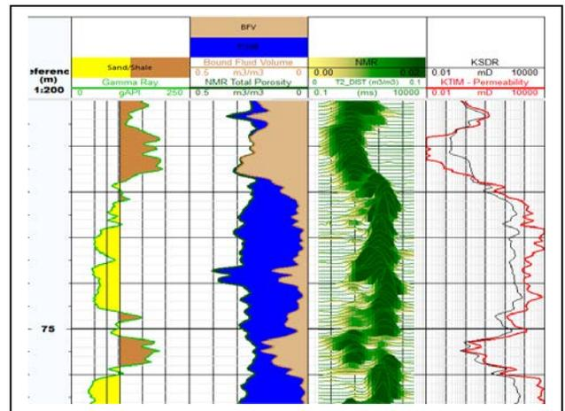
**Figure 6:** Basic NMR log with slimline tool, stacked with natural gamma. Data is inverted to give a continuous T2 distribution for the logged interval (~3 samples/m). T2 distribution readily interrogated to derive total porosity, along with bound fluid (clay and pore bound), free fluid (readily movable), and permeability. Track 3 is the NMR T2 distribution, which represents a pore size distribution (small pores to the left, large pores to the right). (Graphic courtesy of NMRSA Pty Ltd)
