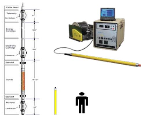
**Figure 5:** New generation slimline NMR tools incorporate oil-field tool design and pulse sequences but smaller and easier to handle in the field, thus opening the door to less expensive field operations. Weight of slimline NMR tools vary with diameter, but generally weigh between 15 and 25 kg. (Graphics courtesy Vista Clara, Inc.)
