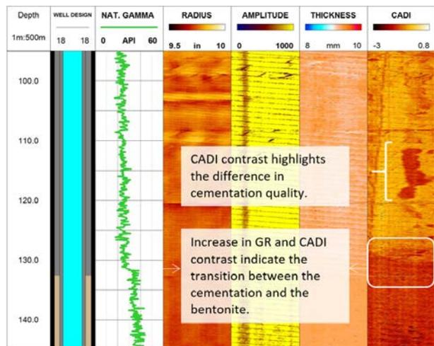
**Figure 4:** Cased hole application in a 20 inch (508 mm) cased well.
