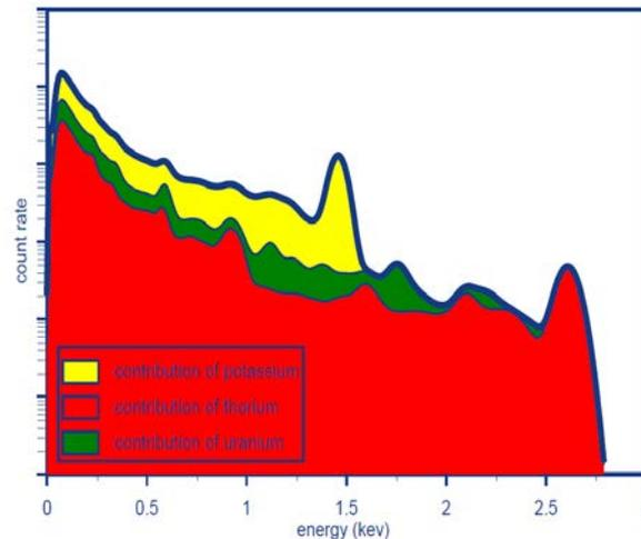
**Figure 10:** FSA of the recorded energy spectrum takes into account the full spectrum (from Limburg and Tijs, 2014).
