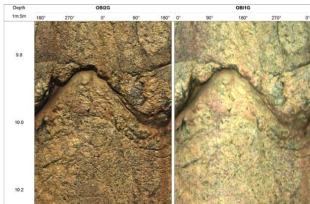
**Figure 1:** Comparing between two different generations of optical borehole imaging tools (QL40 OBI, 1<sup>st</sup> generation, right track) and QL40 OBI 2G, 2<sup>nd</sup> generation, left track) demonstrates the enhanced image quality and resolution that is achievable nowadays with these tools.
