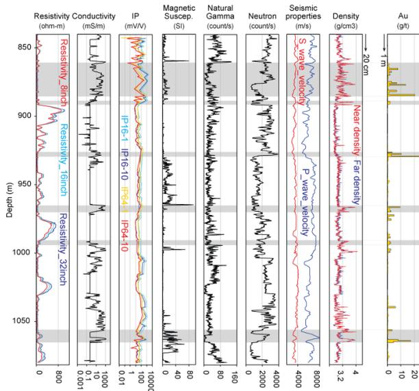
**Figure 1:** Typical geophysical logs at Lalor and gold grades.
