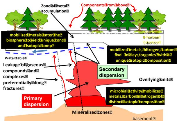
**Figure 2:** Processes involved in primary and secondary dispersion of elements and their isotopes.
