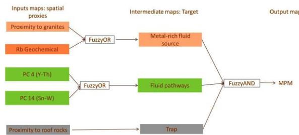
**Figure 2:** Flow diagram of two-staged integration matrix (or inference engine) used to combine the fuzzy evidential maps to produce a resultant mineral prospectivity map (MPM).
