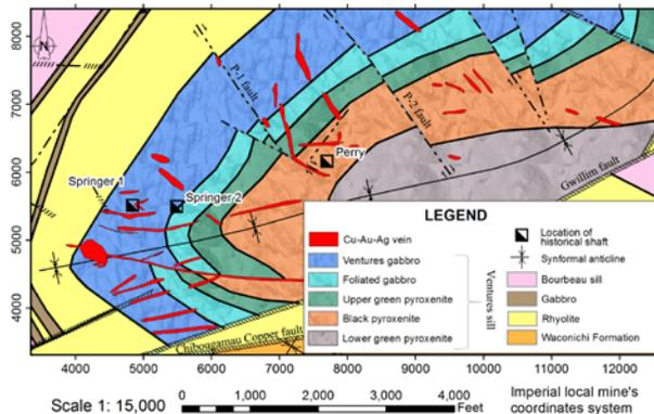
**Figure 1:** Surface geology of the Opemiska area. The location of the historical Springer and Perry shafts are shown. The locations of the Cu-Au veins (in red) are shown at their vertical projection to the surface.
