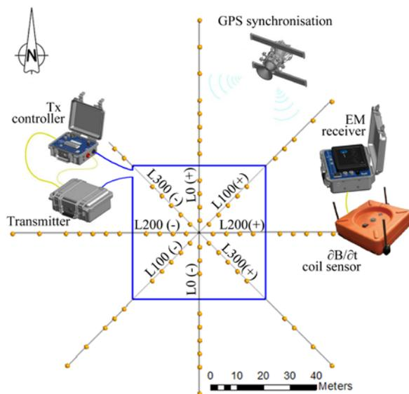
**Figure 4:** Instrumentation set-up for the square fixed-loop transmitter of 50 m side length with the GDD 20 A – 50 V transmitter or with the Geonics TEM 47 transmitter. The line numbering convention is shown in with survey lines radiating from its center at 45° in eight cardinal directions. The x-coordinate is increasing to the north for L0, northeast for L100, east for L200 and southeast for L300.
