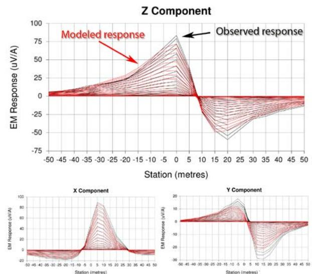
**Figure 5:** Profiles of x, y and z-components, for site #2, L0 from -50 m to +50 m, at 15 Hz, with time windows between 0.08 and 16.484 ms. The observed response is illustrated in black, and the modeled response is illustrated in red.
