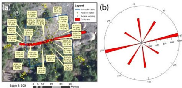
**Figure 8:** (a) Cu-Au-Ag assays for surface dust sampling at site #3 are shown along the vein delineated with a red contour. (b) Rose diagram showing the inverse of the amplitude ratio of the x-component for the time windows 1 and 6 for site #3. Line L200 exhibits the lowest ratio and correspond to the direction of the vein delineated by the red outline.
