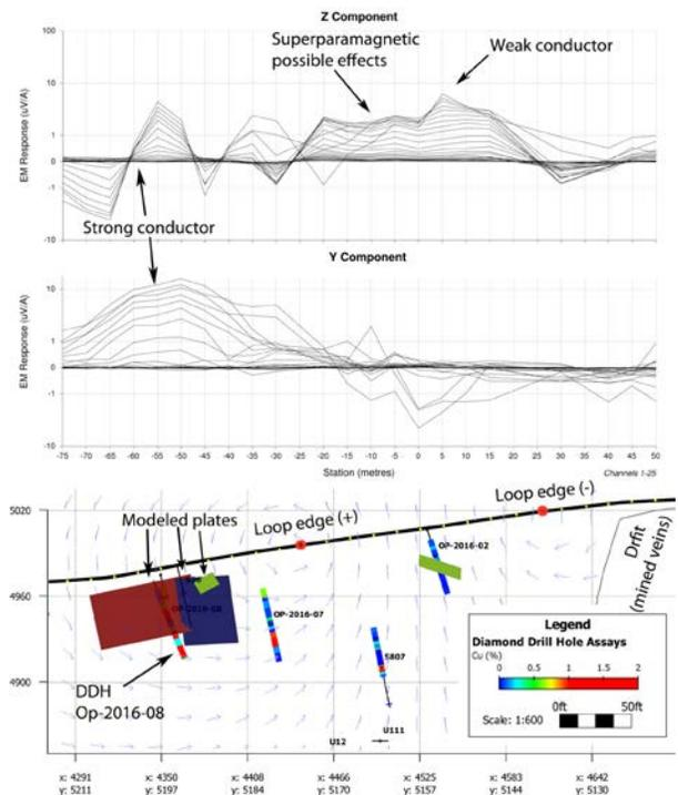
**Figure 7:** Geological longitudinal section (bottom) with drill-hole traces and TDEM profiles (top) along L200 (which follows the vein) of site #4. The modelled plates are shown on the section in red and blue (strong conductance) and green (weak conductance). The primary magnetic field is represented on the section with pale blue arrows, and its polarity is positive inside the loop, with edges at +/- 25 m.
