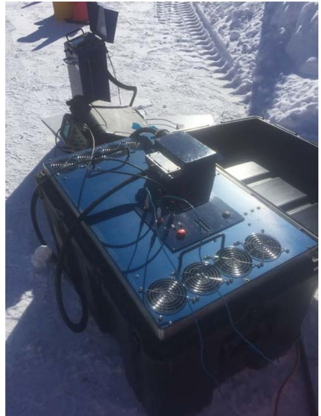
**Figure 2:** UTEM 5 transmitter system, Lamontagne Geophysics Limited.
