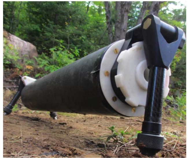
**Figure 5:** UTEM 5 3-component inductive magnetometer sensor (Lamontagne Geophysics Ltd.).
