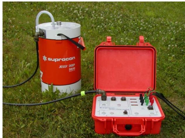
**Figure 3:** Jessy Deep low-temperature 3-component SQUID sensor system (IPHT/Supracon).
