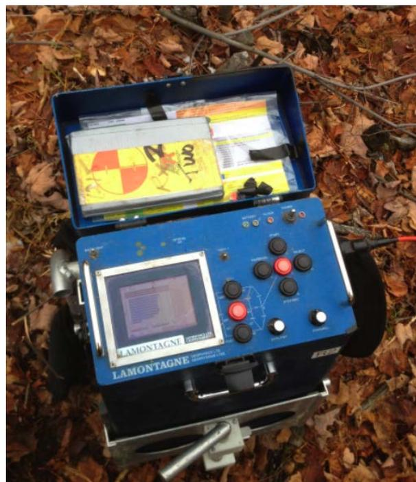
**Figure 7:** UTEM 5 receiver system (Lamontagne Geophysics Ltd.).
