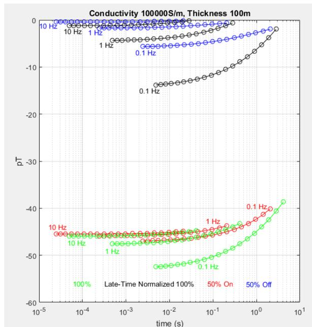
**Figure 15:** Decays calculated for a conductive disc of diameter 200 m, thickness 100 m and conductivity 100,000 S/m. This model is designed to simulate the response of a conductor similar to the Ovoid.
