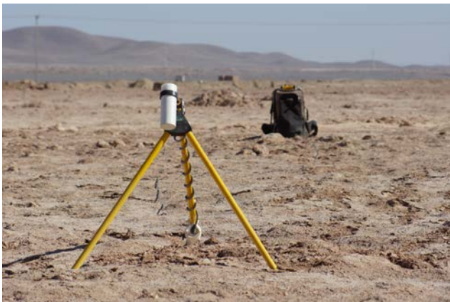
Figure 4: Cesium vapor magnetometer interfaced to a Gap Geophysics frequency counter and data logger system.
