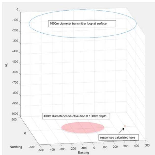
**Figure 10:** Geometry of the model used to simulate the borehole TEM response of highly-conductive targets. The model has a 1000 m diameter circular transmitter loop carrying 20 A current and a 400 m diameter conductive disc at a depth of 1000 m.
