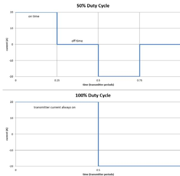
**Figure 11:** Transmitter waveforms used in model calculations.
