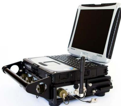
**Figure 6:** SMARTem24 receiver system (Electromagnetic Imaging Technology).
