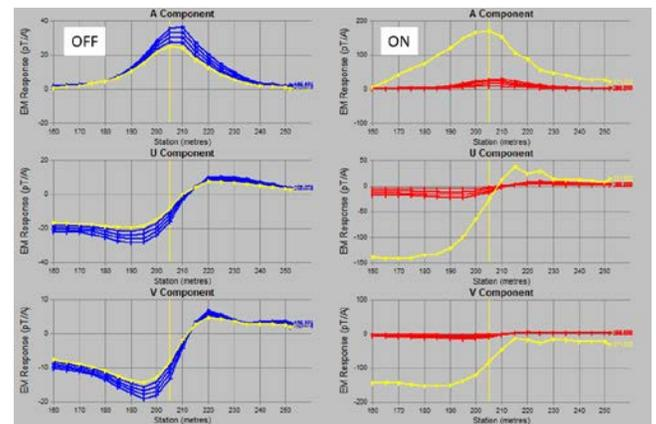
**Figure 24:** Borehole TEM data (0.5 Hz, 50% duty cycle) from adjacent to Moran Deposit, Kambalda. Off-time data on left and late-time-normalized on-time data on right. Time windows from 150 msec onwards.
