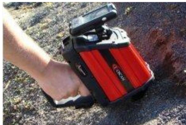
Figure 10: pFTIR spectrometer (photo Agilent).
