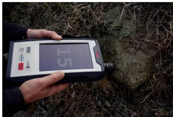
Figure 11:  $\mu\text{Raman}$  spectrometer (photo J. Jehlička).
