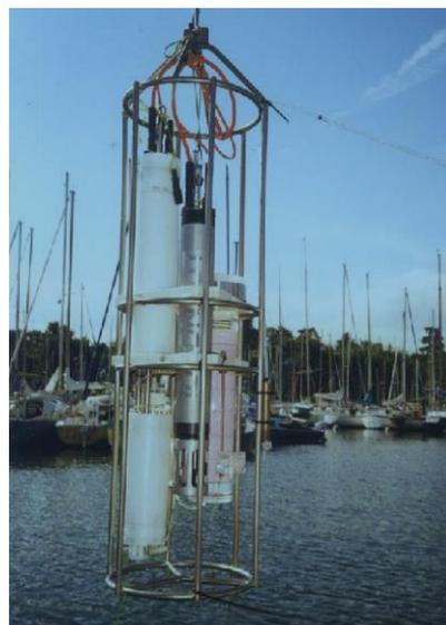
Figure 13: Voltammetric VIP probe (photo Idronaut).
