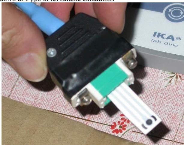
Figure 12: ASV printed electrode.
