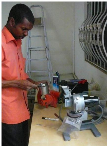
Figure 3: On-site battery-operated sample milling device.
