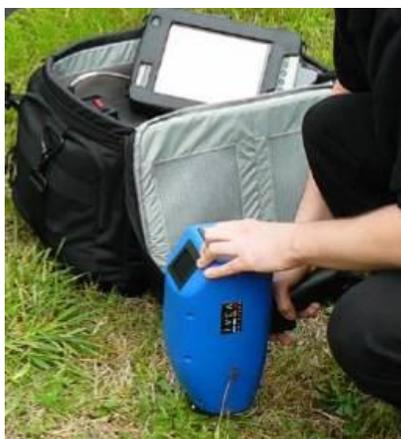
**Figure 8:** LIBS spectrometer (photo IVEA).
