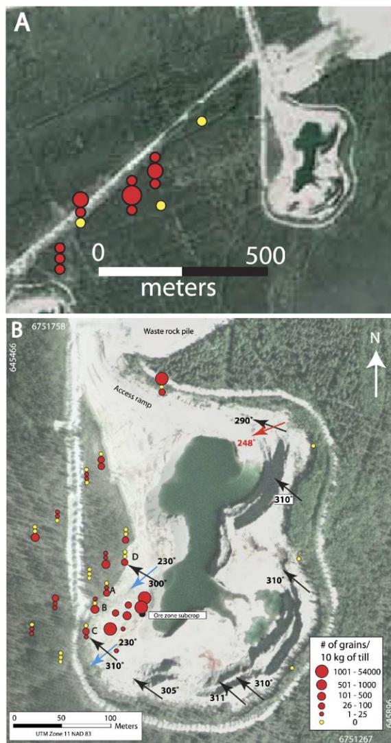
**Figure 5:** Distribution of galena grains in the 0.25–0.5 mm fraction of till samples (A) in the O28 deposit area, and (B) proximal to the O28 ore zone.
