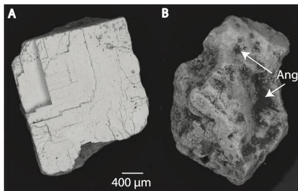
**Figure 6:** Secondary electron images of galena grains from a till sample collected approximately 250 m from ore zone. The grains are cubic (A) to sub-rounded (B). The sub-rounded appearance may be due to the coating of anglesite (Ang) on this grain which is absent from the grain in (A).
