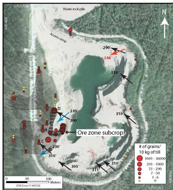
**Figure 4:** Distribution of sphalerite grains in the 0.25–0.5 mm fraction of till. The cross-hatched pattern shows samples that contain sphalerite grains in the 0.5–1.0 mm fraction, and the thick-lined pattern shows samples containing sphalerite grains in the 1.0–2.0 mm fraction that tend to be closer to the orebody.
