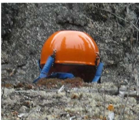
**Figure 1:** Typical deployment of the ELF coils. Approximate diameter is 0.5 m.
