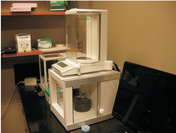
Figure 4: The Immersed Weight ( W_I ) of a sample being measured by suspension in a beaker of water below a balance, using a laboratory-designed Jolly balance.
