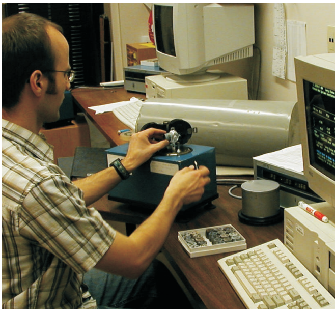
Figure 9: Agico JR5-A Spinner Magnetometer for measuring magnetic remanence.
