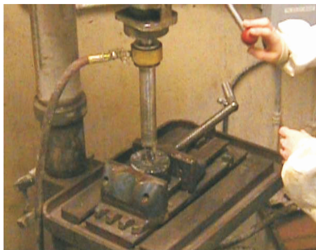
Figure 1: Drilling 2.5 cm diameter subsample cores from a hand sample or exploration core.
