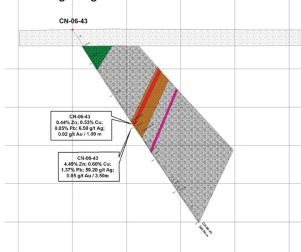
Figure 5: InfiniTEM® survey profile (A) and associated geological cross-section (B) within Coulon Property over survey line 7+00N. Anomaly "EM-01" centered on 0+25W shows the signature of a conductor steeply dipping to the west and buried at a depth of approximately 75 meters. Inferred cross-section from DDH CN-06-43 agrees with qualitative interpretation.
