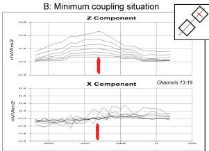
Figure 3: InfiniTEM® survey results over Caber-North deposit (in red) using a loop design of 400 x 400 m half-loops 200 m apart. A: The deposit is located in the area of horizontal primary field yielding in a maximum coupling situation. B: The deposit is located in the area of vertical primary field yielding in a minimal coupling situation. For both cases, the 350 m deep conductor is detected. A Protem 67D and a TEM57 and TEM67 transmitting combo were used to energize the ground with 8 amps.
