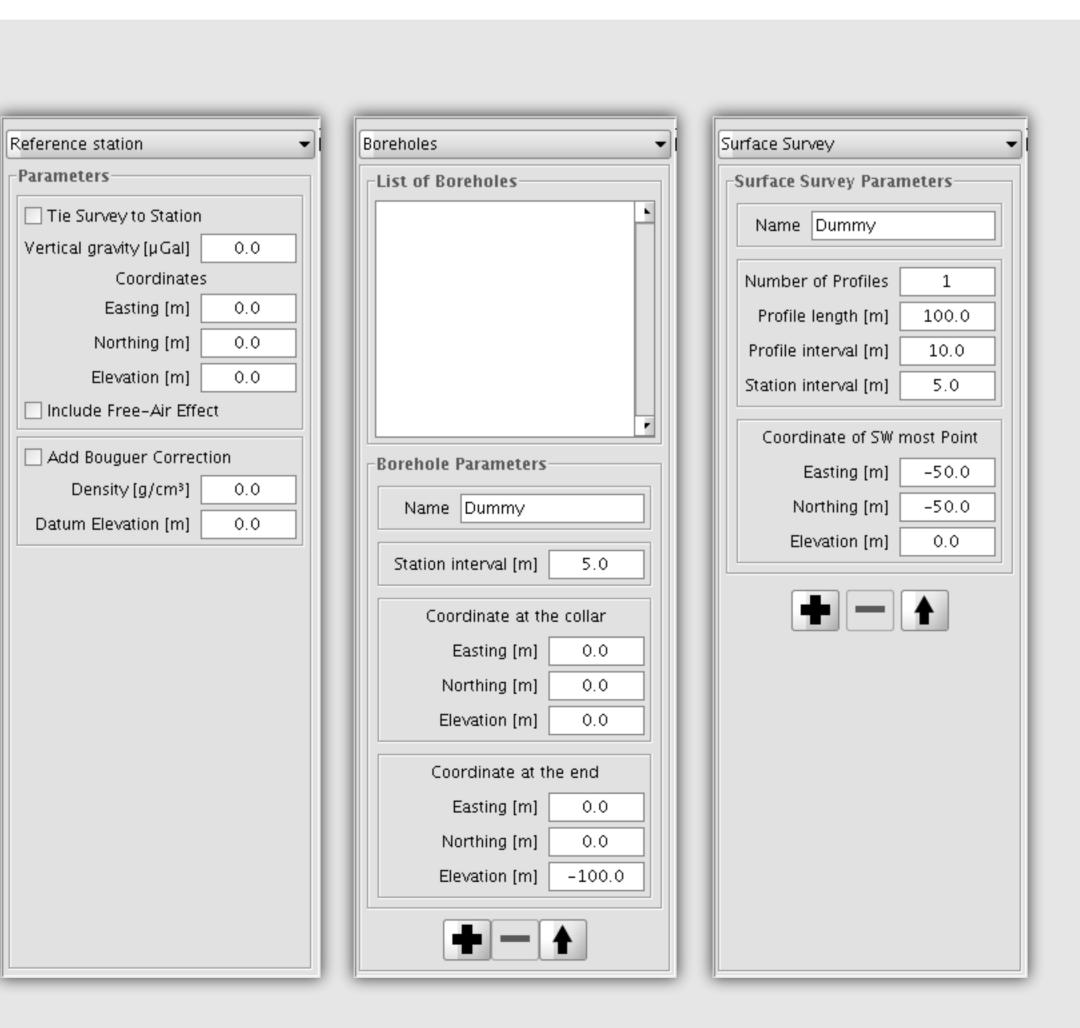
Figure 3 - Panels used to define the survey parameters and station location, and to import field data. It is possible to tie the modeling results with field data at a common reference station. It is also possible to include the Free-Air effect in the modeling, and add a Bouguer correction to the modelled data.
