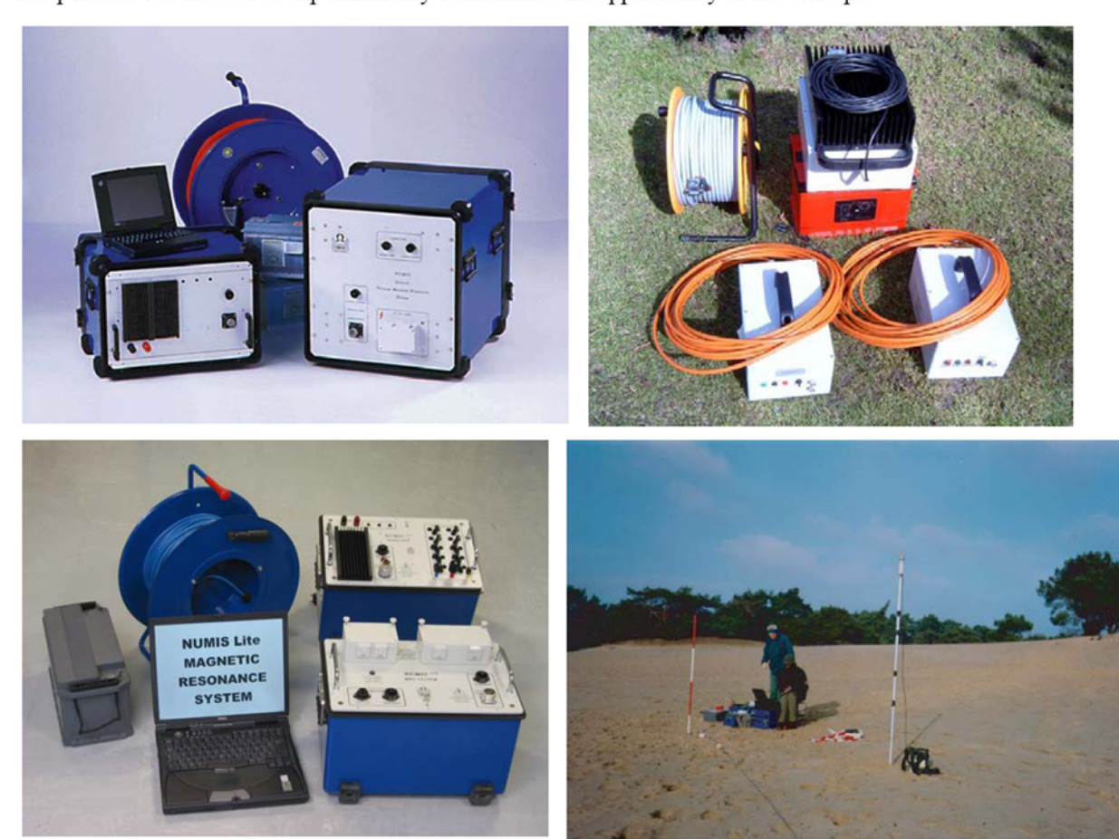
Figure 5: MRS implementations: top left: original NUMIS, top right: Radic SNMR MIDI, bottom left: NUMIS LITE , bottom right: NUMIS plus with EDA magnetometer in monitoring mode at Waalwijk-2.
