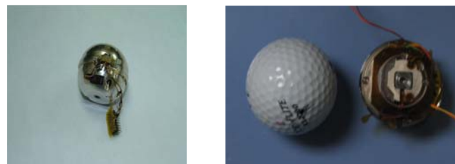
Figure 1: Copper Ball housing the gravity sensor
