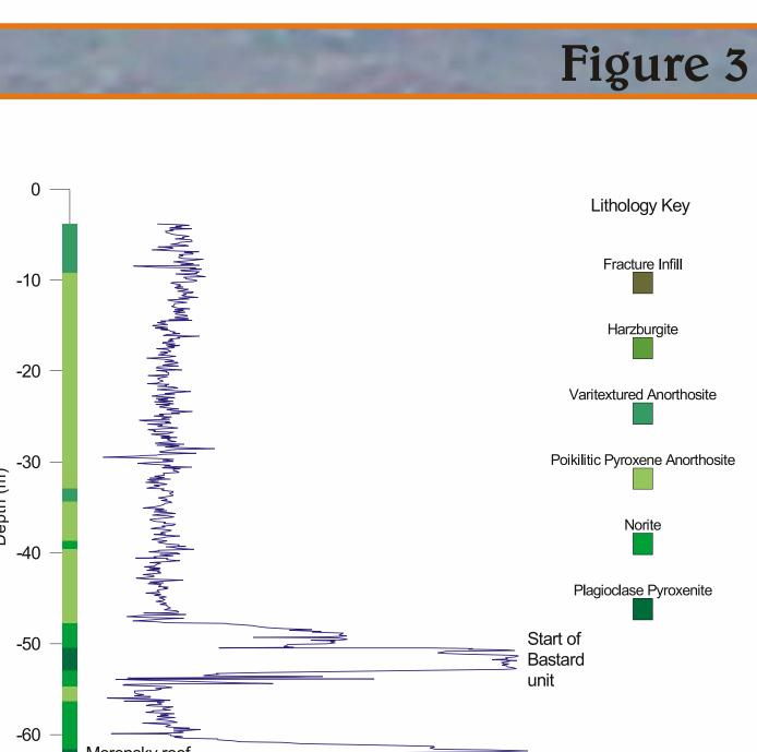
Figure 3: Plots of the individual desity profiles with the simplified geology for comparison. The key given with the Gc10 profile.
