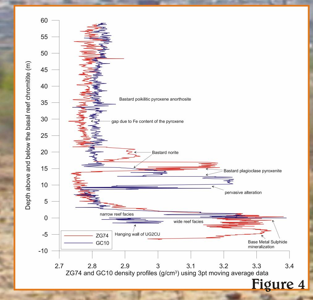
Figure 4: Density comparison between ZG74 (red) and GC10 (blue) showing the close relationships between the two profiles which come from boreholes almost 300km apart. The base line (zero depth value) is the basal reef chromite stringer. The Merensky Reef is seen either as the narrow reef facies or the wide reef facies.
