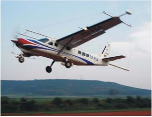
**Figure 3:** The Genesis electromagnetic system mounted on a Cessna 208B, Kakira, Uganda.
