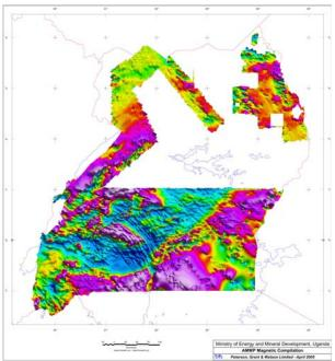
**Figure 1:** Historical geophysical coverage of Uganda, represented by the total magnetic field, shaded from the northeast, compiled by the African Magnetic Mapping Project.
