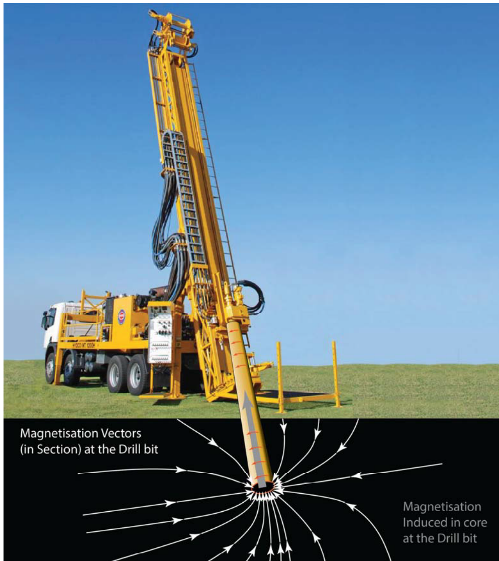
Figure 1: Schematic Illustration of how drilling induced magnetization is acquired.
