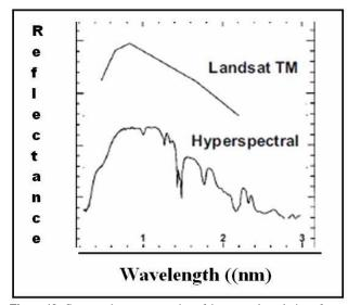
**Figure 19:** Comparative representation of the spectral resolution of satellite-based Landsat versus airborne hyperspectral. The detailed character of the reflectance curves provides discriminatory information for the mineral type. Hyperspectral is therefore potentially a more powerful tool for the categorization of minerals. After .Stevens and Zamudio, undated web publication).
