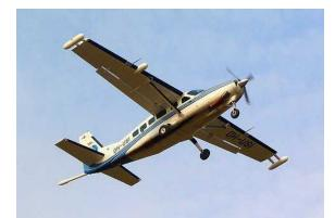
**Figure 9:** A typical fixed wing frequency domain electromagnetic system with wingtip mounted transmitter and receiver pods clearly visible. The tail stinger is not a component of the EM system; it contains a magnetometer. Courtesy of GTK
