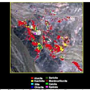
**Figure 21:** Cutout from Figure 17. The resolution of hyperspectral technology can create a detailed suite map of related minerals. After Stevens and Zamudio, undated web publication.
