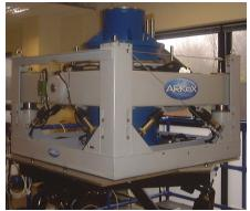
Figure 8: An example of a second generation airborne gravity gradiometer system in a cryogenic dewar (blue cylinder) on shaker table undergoing tests. The vertical dimension of the dewar is about 1.1metres. Courtesy of ARKeX
