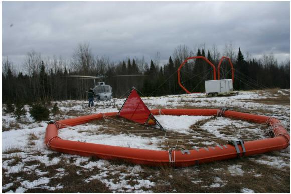
Figure 17: Geotech Ltd.'s AFMAG system showing Z axis receiver in foreground and ground-based monitoring coils in background.
