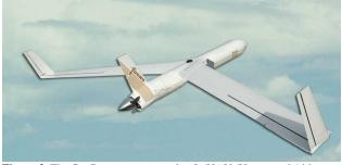
Figure 3: The GeoRanger, an example of a UAV (Unmanned Airborne Vehicle) designed for geophysical application. Courtesy of Fugro Airborne Surveys
