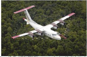
Figure 13: The MEGATEM<sup>™</sup> system was developed for high altitude applications, but also enabled the development of higher power systems as measured by peak dipole moment. Courtesy of Fugro Airborne Surveys
