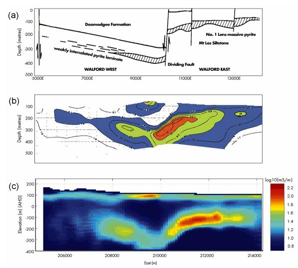
**Figure 18:** Example of a conductivity depth section. (a) Schematic long section, (b) conductivity section based on ground EM, and (c) conductivity section derived from TEMPEST AEM data for 8030100 mN at the Walford Creek Prospect. (a) and (b) are reproduced from Figures 3c and 3b of Webb and Rohrlach (1992). Note that the vertical scale for (a) and (b) is depth below surface, whilst for (c), it is elevation above sea level. After Lane et al, 2000.
