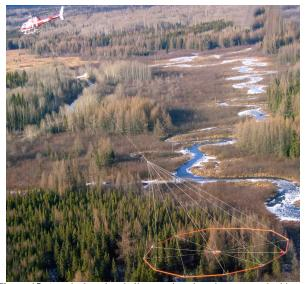
**Figure 15:** A typical modern helicopter time domain system – in this case, VTEM (circa 2004), which used a non-rigid coplanar transmitter-receiver geometry. Courtesy of Geotech Limited
