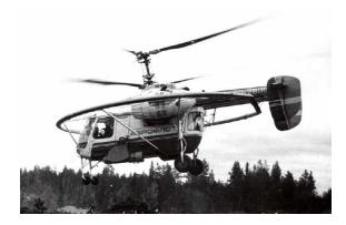
Figure 14: The AMPP-2 is an example of a helicopter time domain system which dates back to the 1970's. Courtesy of Andrey Volkovitskiy
