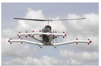
Figure 2: The ORAGS VG-22 system with 11 boom mounted vertical gradiometers (22 total field magnetometers) for UXO detection. Courtesy of Oak Ridge National Laboratory
