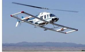
Figure 16: The ORAGS-TEM system developed for unexploded ordinance detection where high near-surface spatial resolution and reliability of detection is required. Courtesy of the Oakridge National Laboratory
