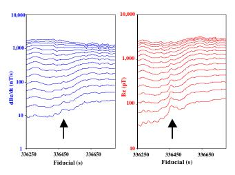
**Figure 12:** Comparison of a dB/dT and a B-field response. The black arrows indicate the position of a massive sulphide conductor. The dB/dT (response on left) and B-field (response on right) data were gathered concurrently. The enhanced late time (lower channels) of the B-field is (are) clearly evident. After Wolfgram and Thomson, 1998.
