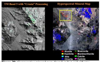
Figure 20: Comparative mineral maps from Landsat and airborne hyperspectral over an area of Chile. The area delineated by the yellow box is shown below. After Stevens and Zamudio, undated web publication.
