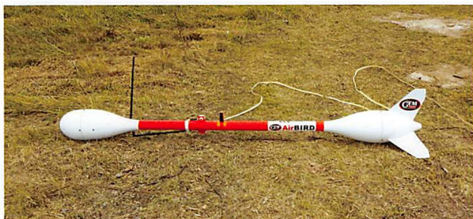
GEM Systems' AirBIRD turnkey light-weight towed-bird magnetometer system designed for UAVs.
