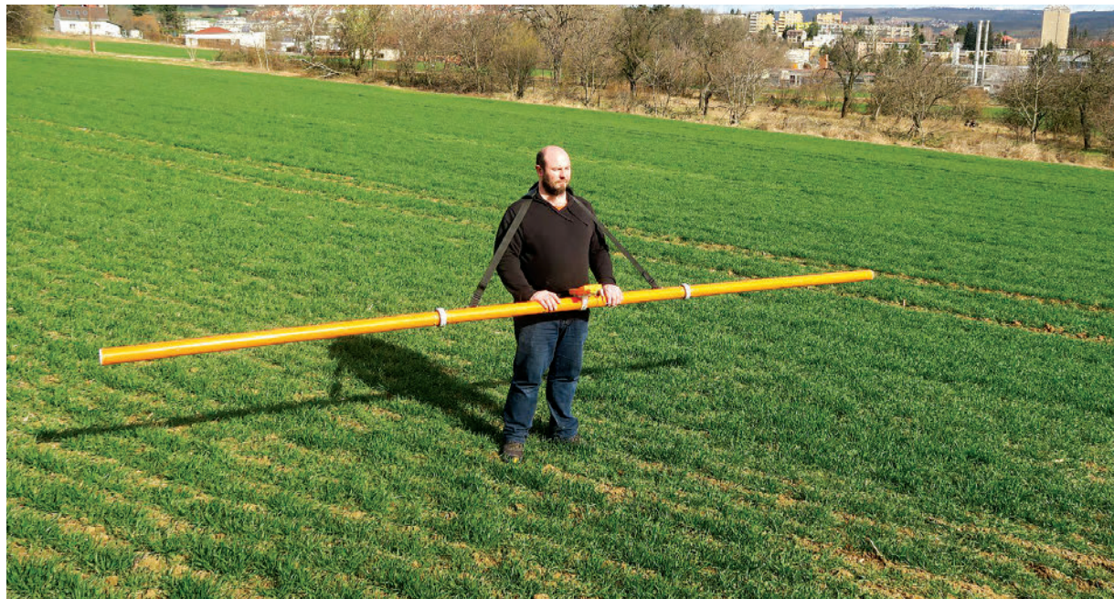
■ GF Instruments' CMD EXPLORER 6L multi-depth probe for EM conductivity measurement (see page 19). Credit: GF Instruments
