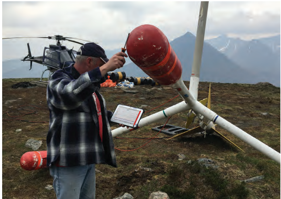
■ Conducting mag sensor pre-survey QC check with SHA Geophysics' wireless DAQNAV 3D system. CREDIT: SHA GEOPHYSICS
