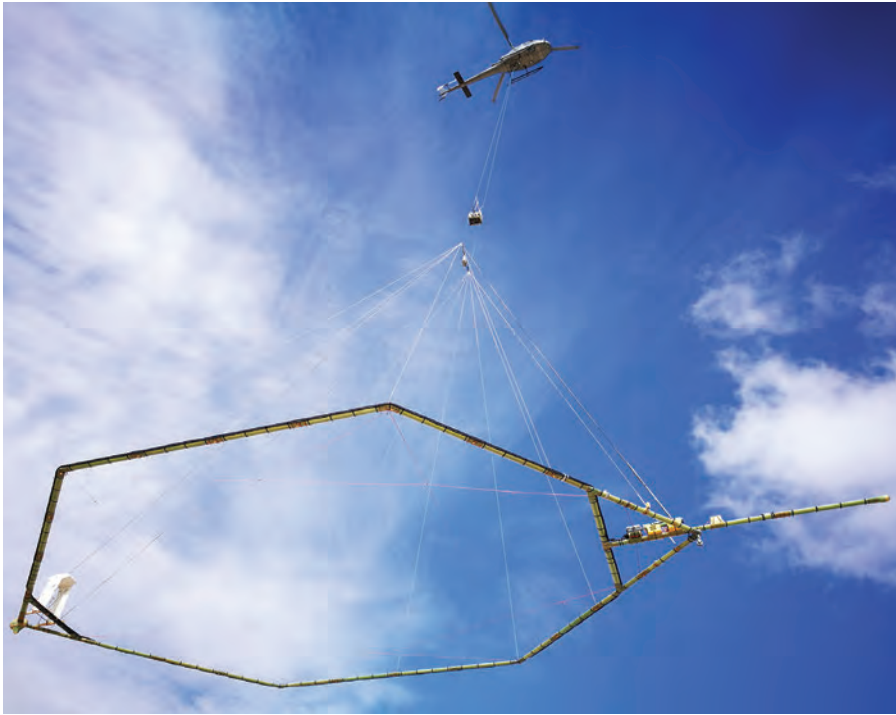
■ SkyTEM Surveys' helicopter and EM loop on survey. CREDIT: SKYTEM CANADA
