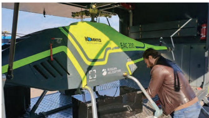
■ Aerogeophysica's strapdown airborne gravimeter in thermal case ready to install on UAV. CREDIT: AEROGEOPHYSICA
