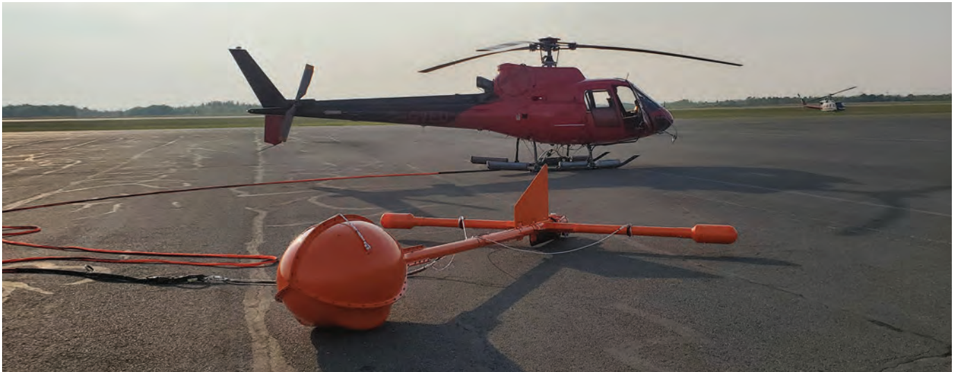
■ Expert Geophysics' newly developed MobileMTm system with horizontal magnetic gradiometer. CREDIT: EXPERTGEOPHYSICS
