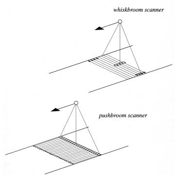
Figure 7: The acquisition geometry of whiskbroom and pushbroom instruments.
