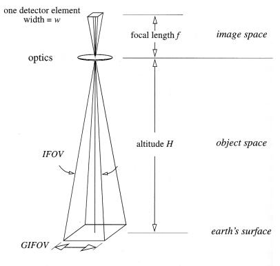
Figure 9: Generalized optical path for remote sensing instruments.
