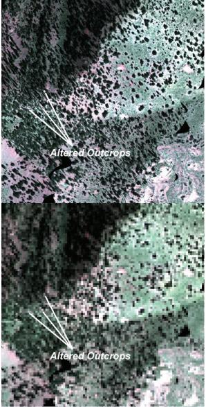
**Figure 11:** Comparison between 1 meter data (top) and 5 meter data (bottom) showing alteration (pink) in a lightly to moderately forested area. Individual altered outcrops that are visible in the 1 meter data are mixed with vegetation in the 5 meter data.
