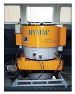
**Figure 3:** The HyMap instrument mounted in a survey aircraft. The lower part of the system is a stabilized platform.
