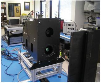
Figure 5: The ProSpecTIR dual HSI camera system (AISA cameras) on a workshop bench
