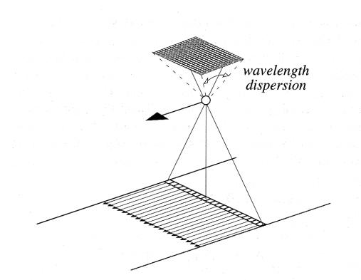
Figure 8: Spatial and spectral acquisition geometry of 2-D pushbroom HSI systems.
