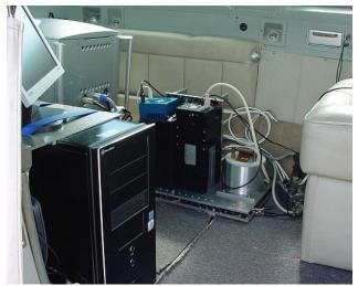
Figure 6. An operational prototype of the HySpex system mounted in an aircraft.
