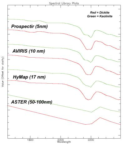
Figure 1: Comparison between the spectra of dickite and kaolinite for the ASTER multispectral instrument and several hyperspectral instruments.
