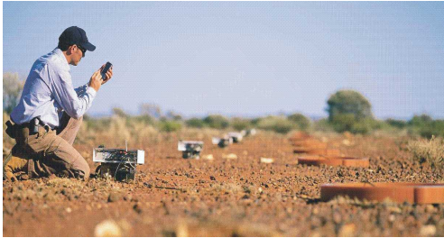
Figure 6: GEOFERRET EM survey showing data acquisition units (left) and sensor coils (right). Data downloaded wirelessly to handheld PC
