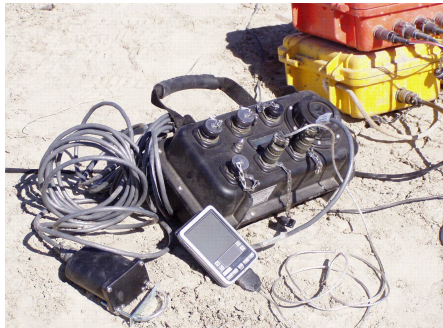
Figure 7: Quantec Geoscience Ltd. six channel acquisition unit for recording multiple electric and magnetic fields simultaneously. Data are downloaded to palm pilot via a serial cable.
