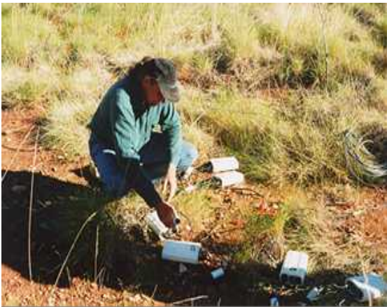
Figure 2: MIMDAS Mark I single channel distributed acquisition units (DAUs). High power-to-weight lithium-ion batteries inside the DAUs powered the electronics.
