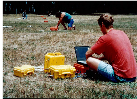
Figure 4: An MT-24 magnetotellurics system being deployed in the field. The original system shared the same core electronics as were developed by Refraction Technology for the MIMDAS system, the RT-120 module.
