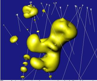
**Figure 4:** An oblique view of an automated grade-shell model created by Leapfrog software. The yellow surface represents ore at a specific cut-off grade. The white lines are drill-holes. The model is approximately 600m by 300m and modelled to a depth of 500m.
