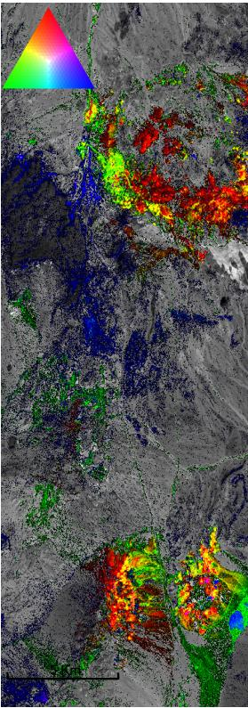
**Figure 18:** Color ratio composite of TM imagery over Goldfield and Cuprite areas in Nevada. RGB are mapped as OH (clay), Iron Oxide, and vegetation/non-altered.
