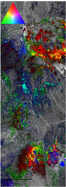
**Figure 19:** Crosta analysis of TM imagery over Goldfield and Cuprite areas in Nevada. RGB are mapped as OH (clay), Iron Oxide, and vegetation/non-altered.
