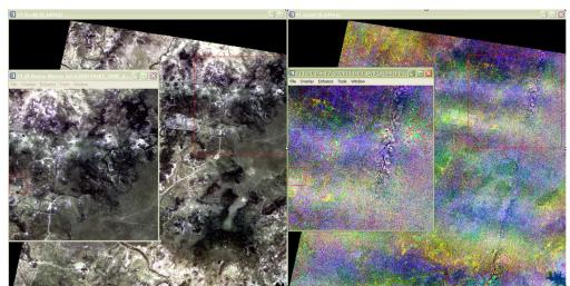
Figure 8: Simple SWIR RGB band display of ASTER image data (left) appears to be without flaws but a processed band ratio image (right) shows an orbit parallel array of noise features produced by a flaw in the ASTER diffraction grating.
