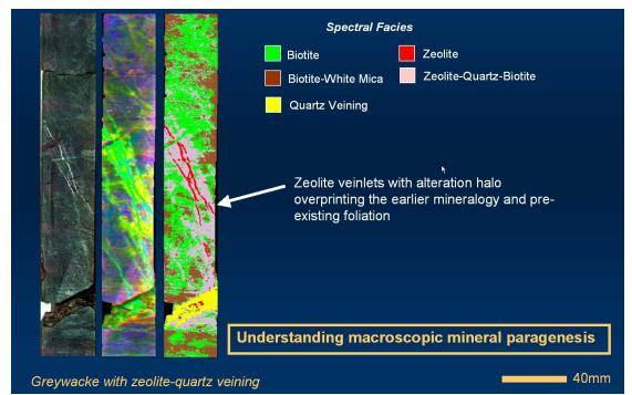
Figure 11: The use of hyperspectral core scanning to understand alteration paragenesis demonstrated in an example using the SpecTerra Core Imaging System operated by Anglo-American (after Harris et al., 2006).
