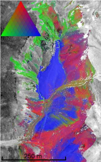
Figure 25: High spatial resolution (1 meter) hyperspectral results for the "Buddintonite Bump" area of Cuprite, Nevada. The image maps alunite, kaolinite, and buddingtonite as RGB. Data where acquired by Spectir LLC. using an AISA Dual imaging spectrometer.
