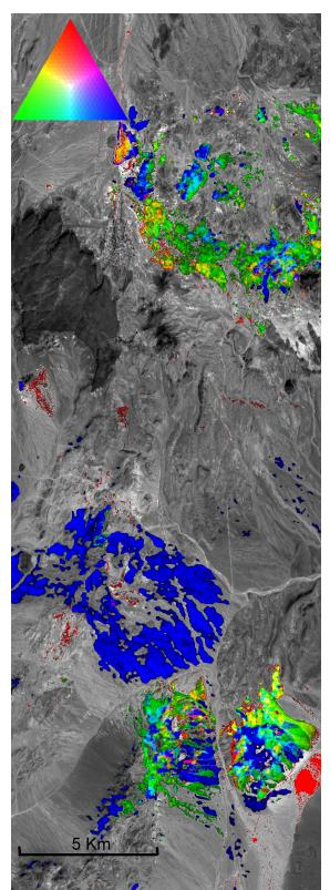
Figure 21: Results of ASTER analysis for the Goldfield and Cuprite areas in Nevada. The image maps iron oxide, clay, and quartz responses as RGB.
