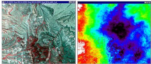
**Figure 5:** AVIRIS Color Infrared Composite image, Bands 52, 33, and 19 (0.85, 0.67, and 0.55 µm) (RGB)(left) and corresponding color-coded water vapor image (right). The color scale goes from black to blue, to green, to yellow, to red, to white (low column water vapor to high column water vapor). Lower water vapor corresponds with higher elevation areas (after Kruse, 1998).
