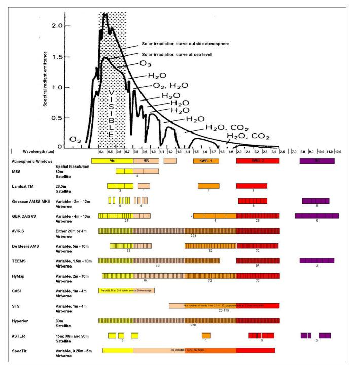
Figure 2: The spatial resolution and spectral band positions of selected sensors plotted relative to incoming solar irradiation, atmospheric absorption and windows.
