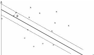
Figure 15: A quality measurement for SVM classification. The simple geometry of the SVM hyperplane (in this case a line) allows the distance to the partition to be easily calculated. In this example one might say that points that fall within distance g from the partition could belong to either class "x" or "o".
