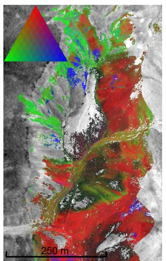
Figure 24: High spatial resolution (1 meter) hyperspectral results for the "Buddintonite Bump" area of Cuprite, Nevada. The image maps alunite, kaolinite, and illite as RGB. Data where acquired by Spectir LLC. Using a AISA Dual imaging spectrometer.
