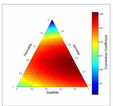
**Figure 16:** Objective function for partial unmixing of iron minerals. The correlation maximum is at approximately 35% jarosite and 65% goethite. This illustrates that the function is smooth and well behaved producing a fast and reliable optimization.
