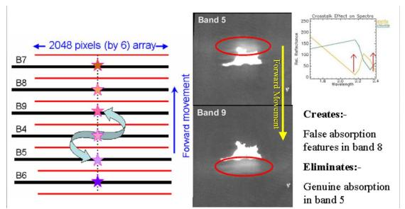
**Figure 7:** Schematic illustration of the "Crosstalk" problem in ASTER showing the spillover or leakage of energy from detector 4 into detectors 5 and 9 relative to the forward motion of the sensor (left), the visual impact on the image demonstrated by the "ghosting" effects in bands 5 and 9 relative to the sensor motion (centre) and the spectral effects of eliminating real absorption in band 5 and creating false absorption in bands 6 and 8 (right).
