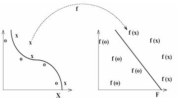
Figure 14: The SVM concept. The transformation (via a kernel function) of non-linearly separable data may allow linear separation (from Christianini, 2001).
