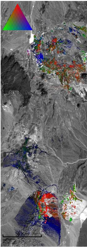
Figure 22: AVIRIS unmixing results (OCCM) for the Goldfield and Cuprite areas in Nevada. The image shows alunite, kaolinite, and illite as RGB.
