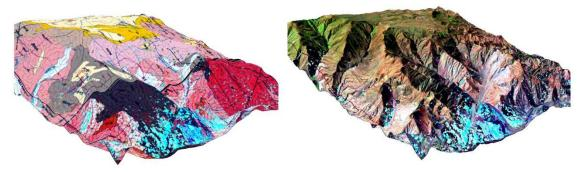
Figure 9: ASTER derived DTM used to generate 3-D visulaisations of phyllic alteration (light blue) relative to mapped geology (left) and standard image algorithms (right).
