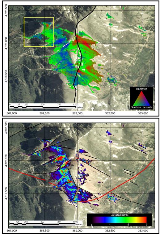
**Figure 13:** Partial unmixing results for iron minerals from hyperspectral data in the Grizzly Peak Caldera. The image is of a developing leach cap over an unexploited Mo-Cu porphyry. The top image maps hematite, goethite, and jarosite as RGB. The bottom image is the jarosite/goethite ratio calculated from the partial unmixing image.
