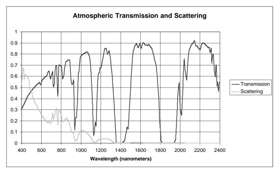
Figure 12: Atmospheric transmission and scattering.
