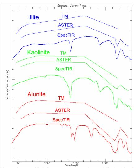
Figure 1: Comparisons of the spectral signatures of alunite, kaolinite, and illite as measured by the TM, ASTER, and SpecTIR sensors.
