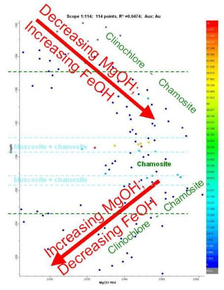
Figure 10: ASD Terraspec analysis of drill core from the Jundee gold mine, Western Australia showing the increase in chlorite absorption wavelength and hence FeOH content relative to MgOH towards mineralization in both the hanging wall and footwall. Colour scale relates to gold grade.
