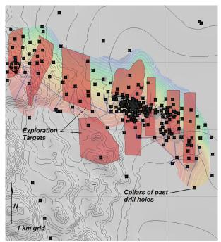
**Figure 4:** Map view of topography and subsurface composite 3D data. Target areas (red) superimposed on structure contour of HW Op contact surface. Collars of drill holes (black squares) show
