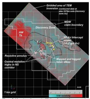
**Figure 5:** Map view of composite 3D data. Large scale conceptual targets based on 3D inversion of TEM data (slice at mid drill hole elevation), the Midway gold zone and mapped rhyolite dikes within the range front.
