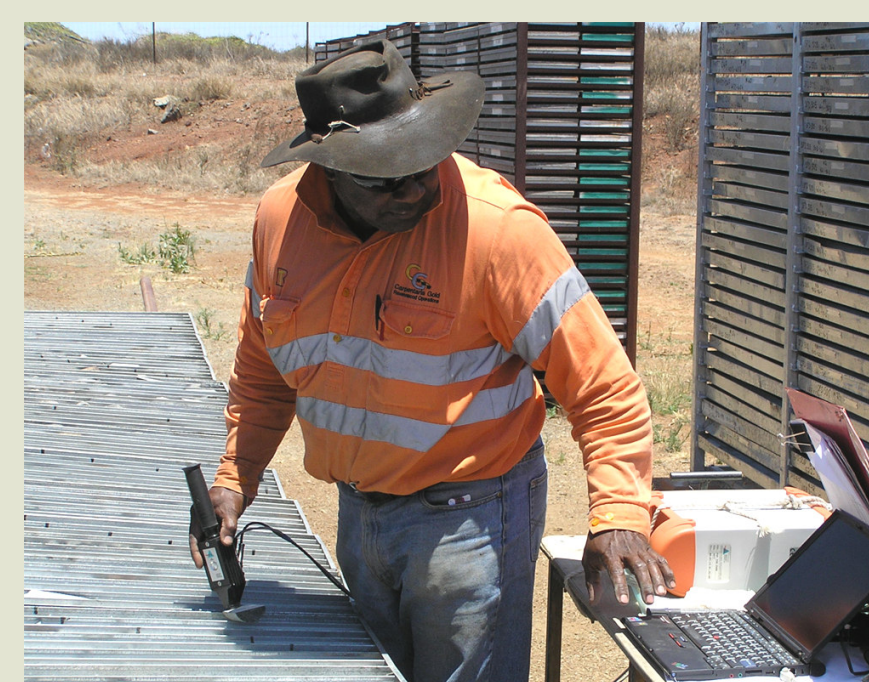
Collection of spectral data with ASD TerraSpec
