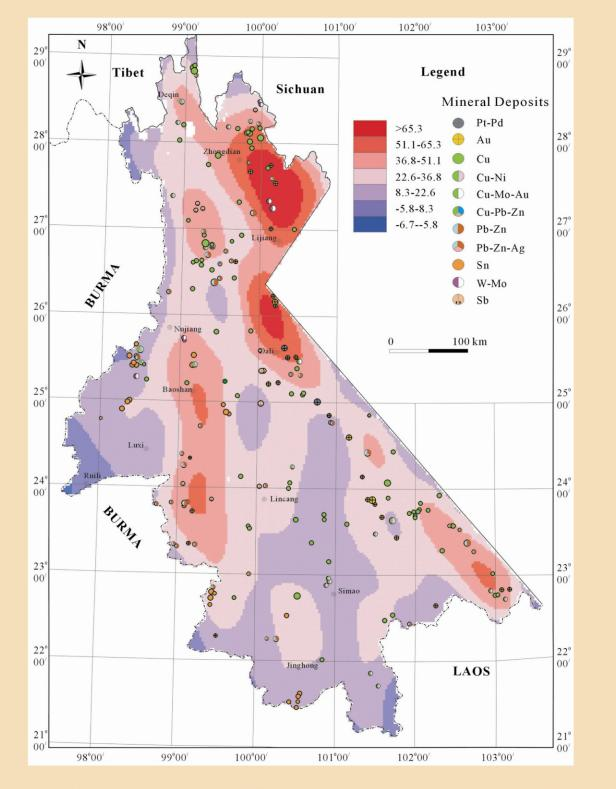
Fig. 4. Regional background component of Cu decomposed from the Cu power spectrum density using IFT with regional background filter as defined in Fig. 3
