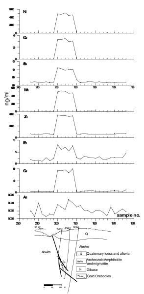
Figure 2: Elemental distributions of geogas in line 220 over Zhangquanzhuang gold deposit, Hebei.
