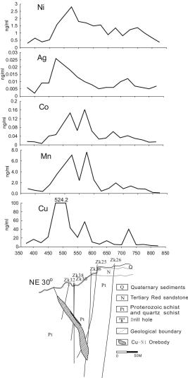
Figure 3: Elemental distributions of geogas in line 204 over Lashuixia Ni(Cu) deposit, Qinghai.
