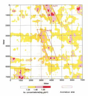
Figure 4: Contour map of log-transformed As concentration in soil for the reconnaissance survey.
