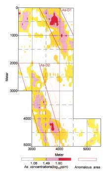
Figure 6: Contour map of log-transformed As concentration in soil for the detailed survey.
