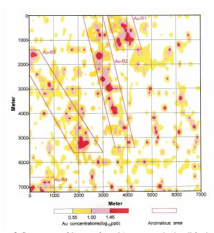
Figure 3: Contour map of log-transformed Au concentration in soil for the reconnaissance survey
