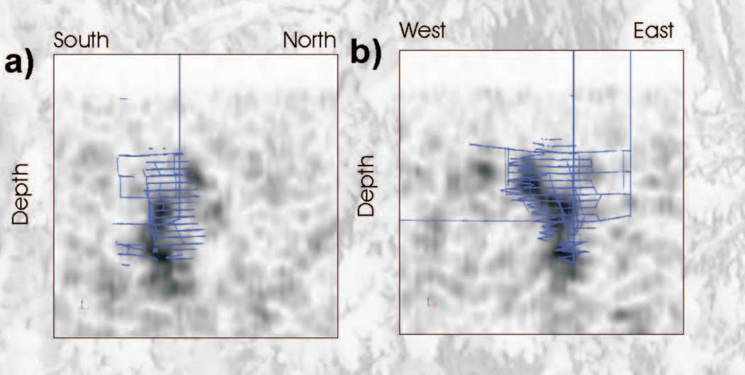
3-D seismic response in the Louvicourt mine.
