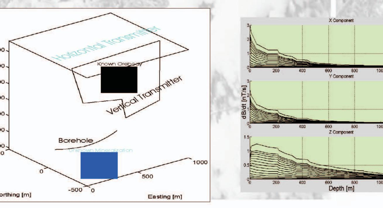
Brown field exploration scenario: BHEM response of the unknown mineralization is masked by responses of the orebody (long wavelength) and stringer sulfides zones close to the borehole (spikes). The left panel of the figure shows the response of the
