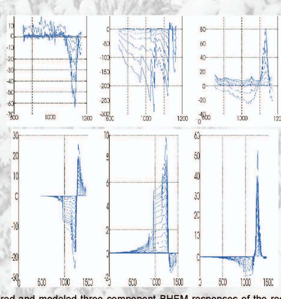
Measured and modeled three component BHEM responses of the red plate amplitudes and decay are matched very well.
