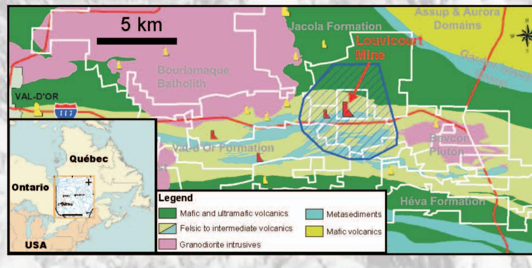
). The 15.5 Mt Louvicourt orebody is a polymetallic (Cu-Zn-Au-Ag) VMS type deposit that depths of 355 and 920 m. The 3-D seismic survey acquired at the Louvicourt mine is shown by the blue hatched area.
