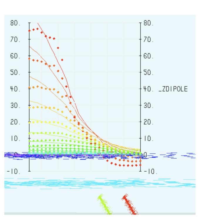
Fig. 9:The effect of a 1-ohm resistance lake.
