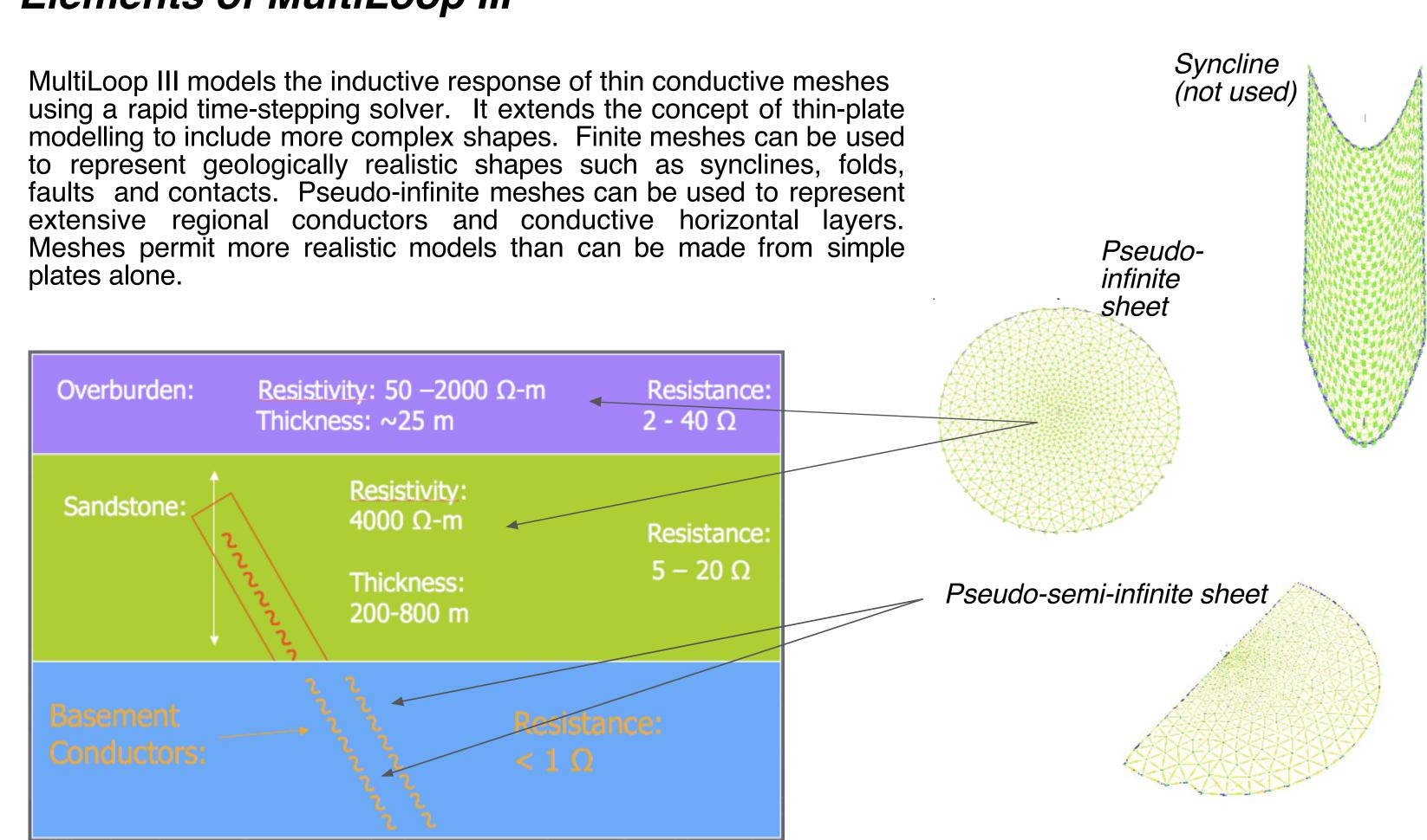
In the Millenium model, the overburden and sandstone were represented by pseudo-infinite meshes, while the basement conductors were represented by pseudo-infinite halfsheets.
