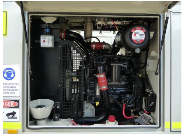
Fig. 5. The HPTX-80 engine compartment showing the Cummins turbo-diesel engine and high capacity radiator. The fuel tank is located beneath the radiator.
