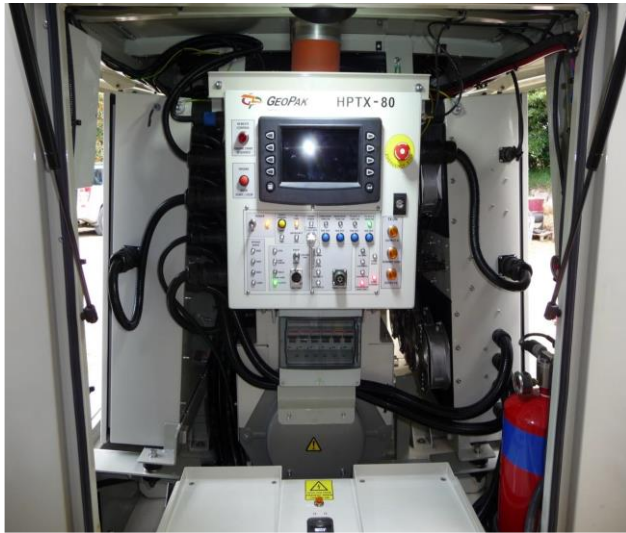
Fig. 6. Rear view of the HPTX-80 with the rear door open showing the grey alternator, control module at top and capacitor box at the bottom. The switch module is located on the left side. The transmitter module is located on the right.
