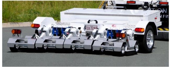
Figure 4: Noise-modulated GPR used for pavement analysis and utilities detection in Australia (Radar Portal Surveys Pty).
