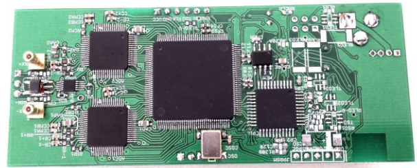
Figure 10: Single-board GPR receiver, control unit and data logger with on-board GPS.
