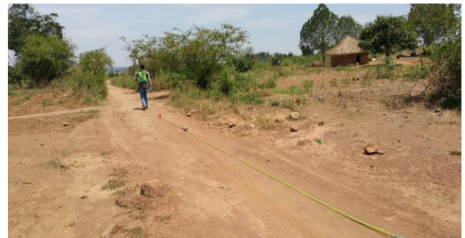
Figure 11: 30 MHz UltraGPR with collinear antennas for rapid surveying in difficult terrain.
