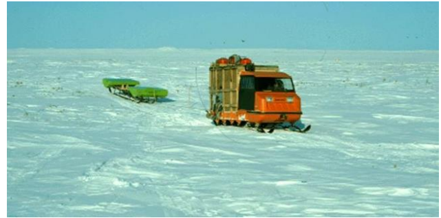
Figure 2: Early GPR system being used to map subsurface conditions along proposed pipeline route.
