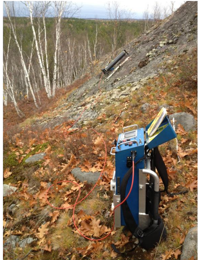
Figure 13: A UTEM 5 receiver mounted on its packframe with tripod legs connected to the UTEM 5 sensor in hilly terrain.
