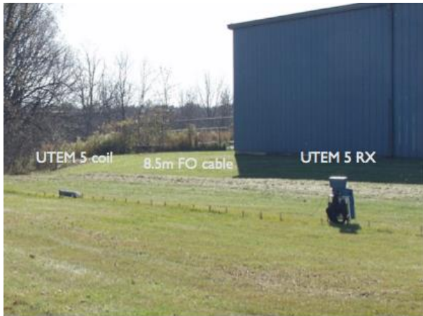
Figure 10: UTEM 5 surface sensor and receiver layout along a test line. To minimize noise due to operator motion the two instruments are set >8m apart.
