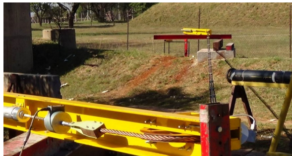
Figure 5: Loop cable and ropes for bird strike tests.
