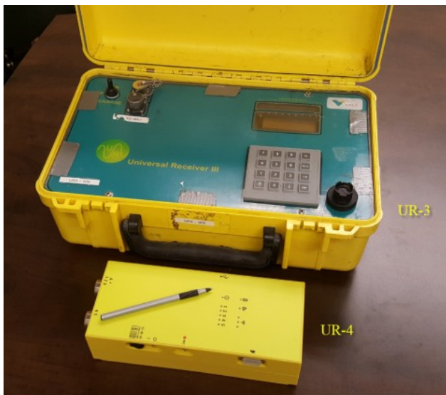
Figure 11: Comparison of the UR-3 and UR-4 receivers.
