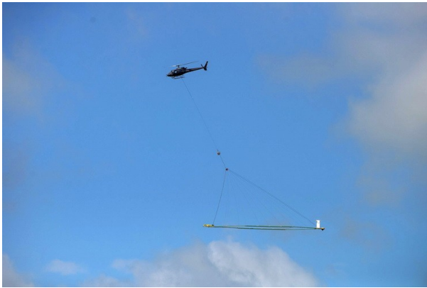
Figure 2. The Fast Flying SkyTEM System at a speed of 150 km/h.
