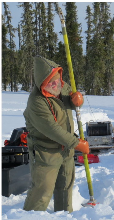
Figure 1: Volterra borehole probe in Northern Saskatchewan. Multiple sections consisting of data acquisition units, battery pack, B-field coil, and 3-component fluxgate magnetometer.
