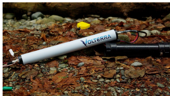
Figure 1: Volterra acquisition unit (surface) with battery pack. Approximate size is 40.5 cm long and 43 mm in diameter
